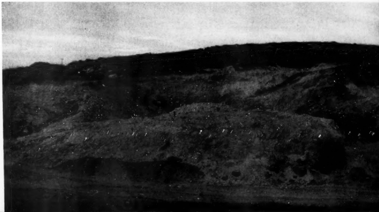
Overburden has been stripped away, exposing the dome-shaped sulphur orebody. The overburden is largely travertine.
